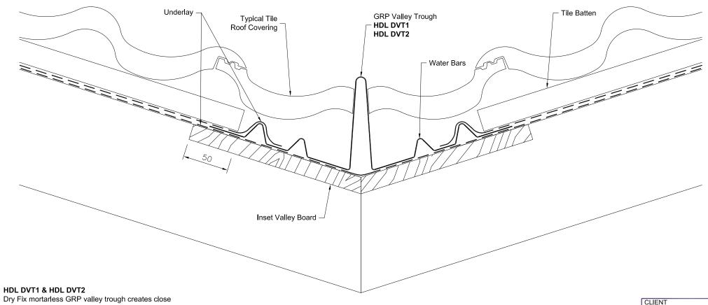
cut appearance on new build and refurbishment. Suitable for all profiled tiles. Available in standard lead grey colour.
